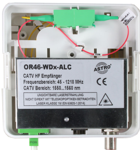
Figure 11: Middle part of the housing with RF receiver
