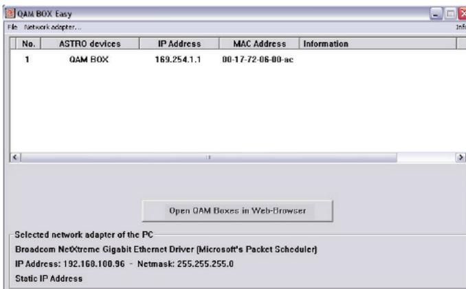
As soon as the process has finished, the MAC- and IP-addresses of the detected modules are listed in a table.
