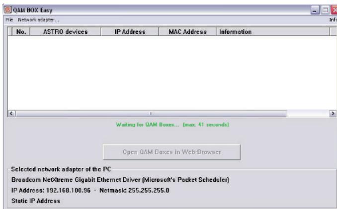
Now start the QAM BOX Easy program installed before. You should now see the starting window of the program (see on the left). The IP addresses of connected QAM BOX modules are now detected automatically. The time remaining until the end of detection is displayed in green color.
